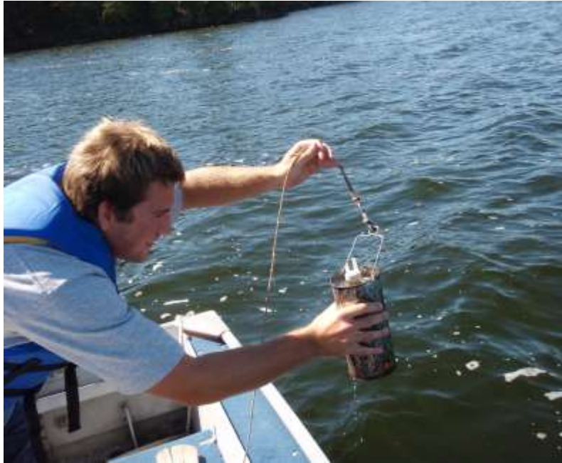
A Composite Sampler (pictured above) is used by dropping the tin container into the water. When it reaches the required depth it is slowly pulled back to the surface. The tin is filled as water enters one tube and air escapes the other. Some air remains in the tin to ensure collection throughout the haul to the surface.
